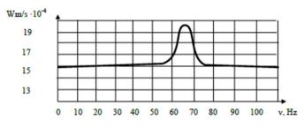
Figure 5: Dependence of the filtration speed on the frequency of oscillations introduced into the solution
